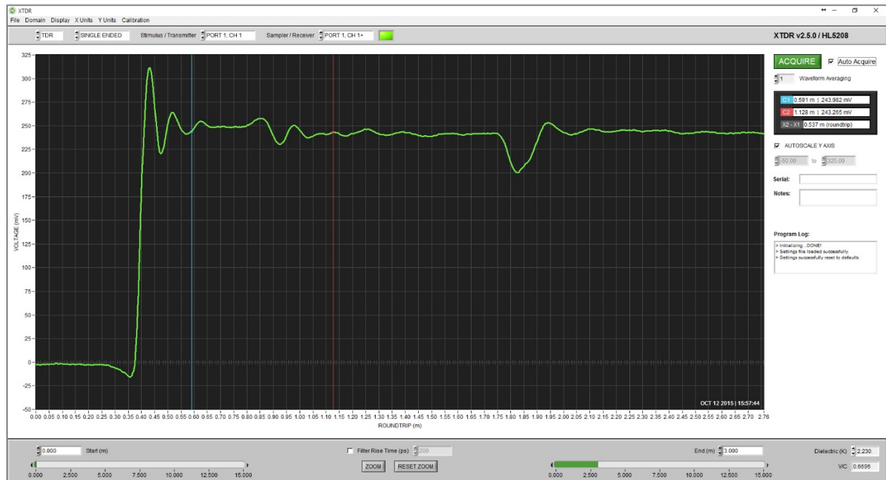
Figure 1: XTDR™ startup screen after initialization and calibration (units in meters, mV)
