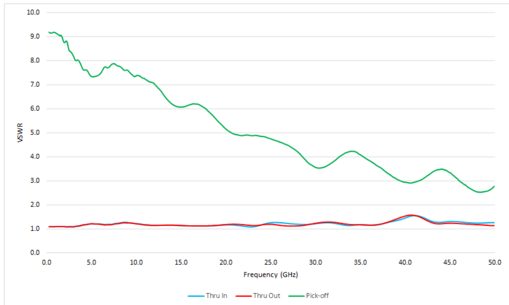
Figure 11: Typical HL9565-U-20-JJJ VSWR on all ports
