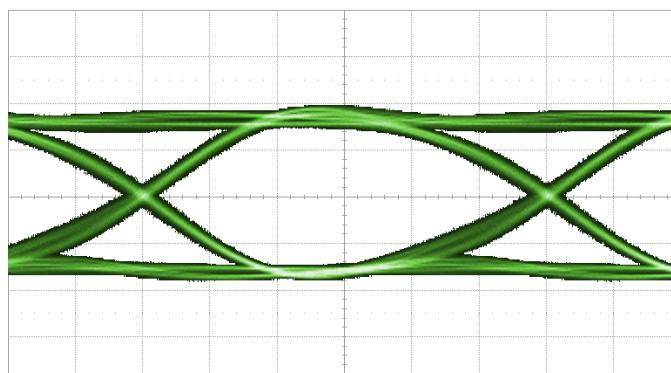
Fig. 10: 24 Gbps PRBS7 pattern on RF Out, 325mV/div.
