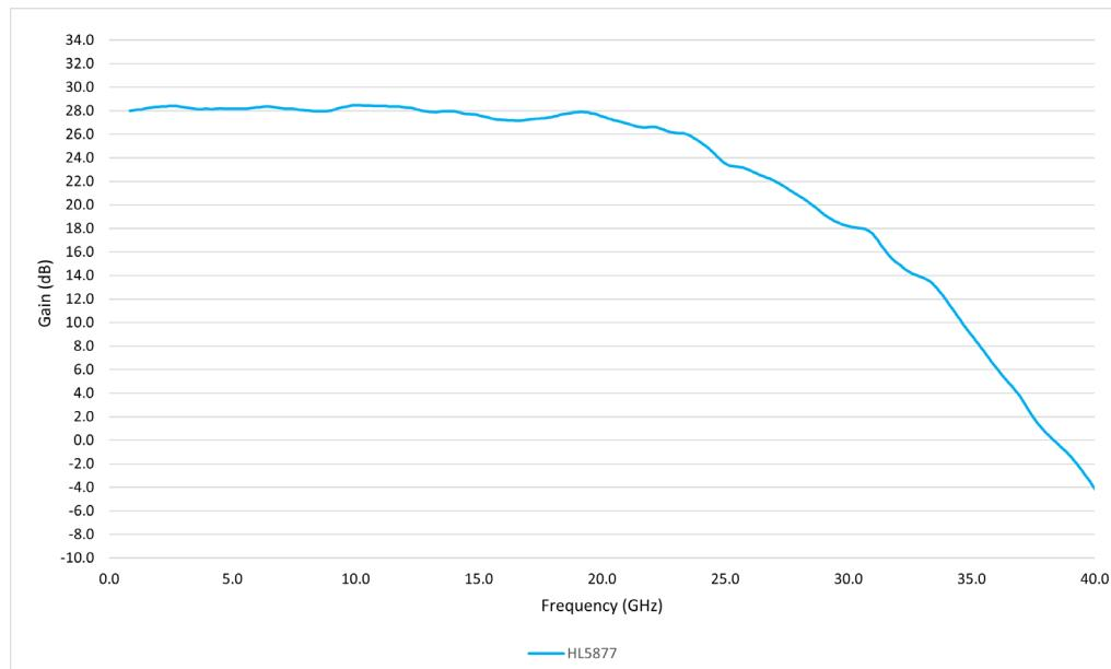
Figure 1: HL5877 Gain (opt. -29-JJ),  $P_{in} = -30 \text{ dBm}$
