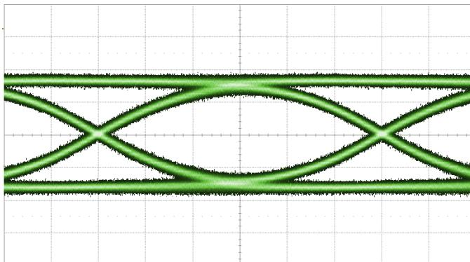
Fig. 7: 24 Gbps PRBS7 pattern on RF In, 30mV/div.
