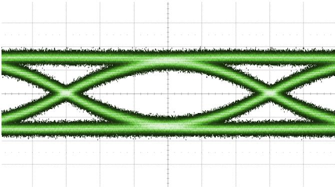
Fig. 5: 24 Gbps PRBS7 pattern on RF In, 16mV/div.
