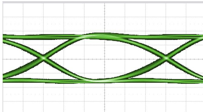
Fig. 8: 24 Gbps PRBS7 pattern on RF Out, 325mV/div.
