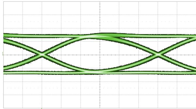
Fig. 6: 24 Gbps PRBS7 pattern on RF Out, 325mV/div.
