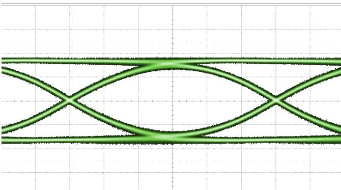
Fig. 9: 24 Gbps PRBS7 pattern on RF In, 260mV/div
