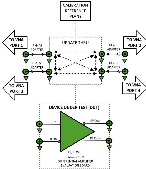
Figure 6: Block Diagram of 4-Port VNA Measurement System
