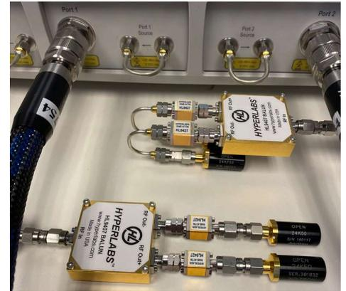
Figure 2: Open Reflect Cal of Port 1
