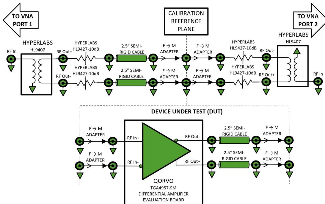
Figure 1: Block Diagram of 2-Port VNA Measurement System Utilizing Two HL9407 Baluns
