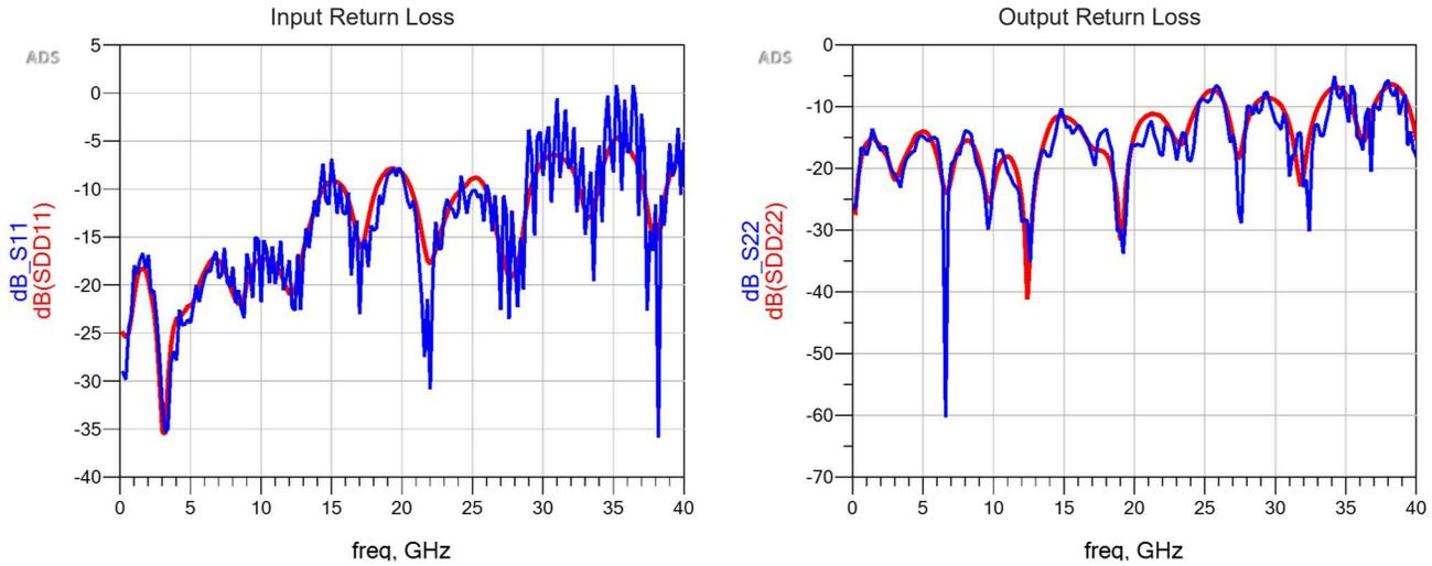
Figure 8: Comparison of Raw Return Loss Data
