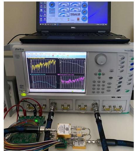
Figure 4: Active 4-port Measurement
