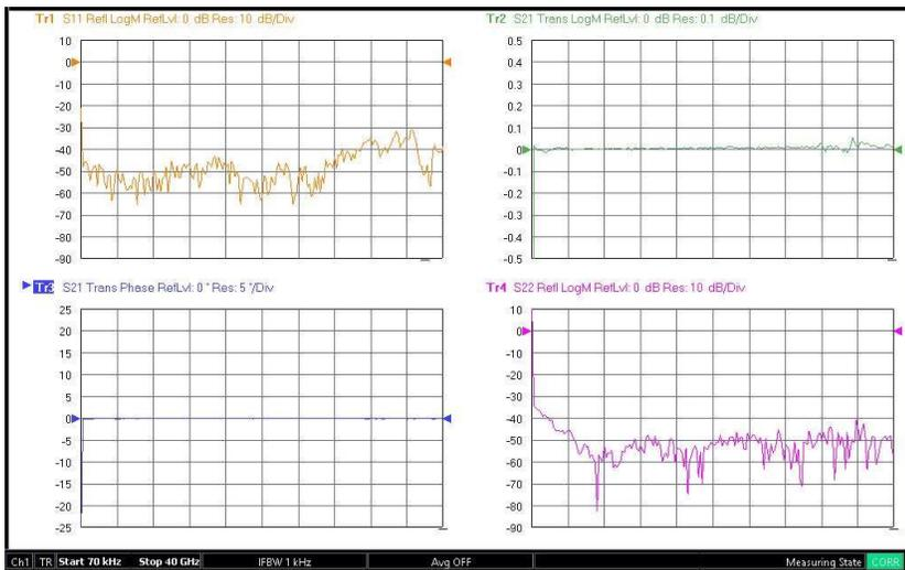
Figure 3: Thru Verification of Differential Calibration
